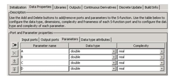
The S-function parameters pane at the top of the S-Function Builder contains the actual values for the state-space matrices, entered as MATLAB expressions. In this example, each state-space parameter is a two-by-two matrix. Alternatively, you can store the state-space matrices in variables in the MATLAB workspace and enter the variable names into the Value field for each parameter.
