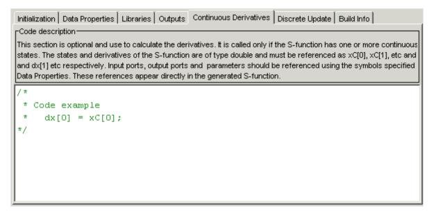
Enter code to compute the derivatives of the continuous states in the **Code for the mdlDerivatives function** field on this pane. When generating code, the S-Function Builder takes the code in this pane and inserts it in a wrapper function of the form
