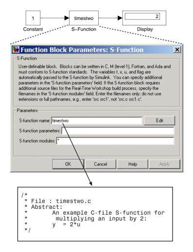
In this example, the model contains an S-Function block that references an instance of the C MEX file for the S-function timestwo.c.
