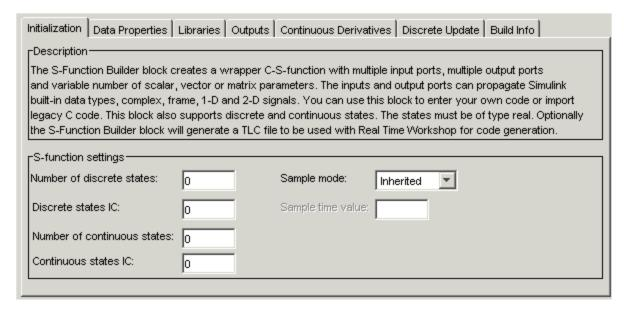
The S-Function Builder uses the information that you enter on this pane to generate the mdlInitializeSizes callback method. The Simulink engine invokes this method during the model initialization phase of the simulation to obtain basic information about the S-function. (See "How the Simulink Engine Interacts with C S-Functions" on page 4-77 for more information on the model initialization phase.)
